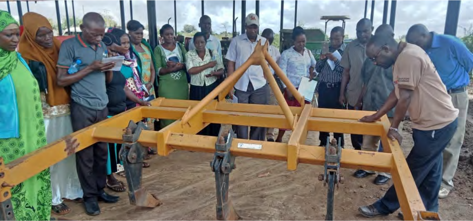
The team viewing a Tractor drawn ripper at the Agricultural Mechanization Service, Wote, Makueni County, Kenya.
